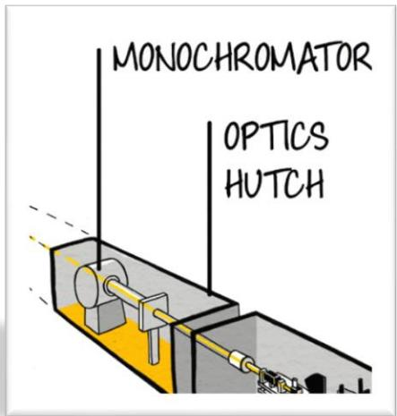
The **monochromator** selects “one” wavelength/energy from the broad band radiation generated by the SR source
