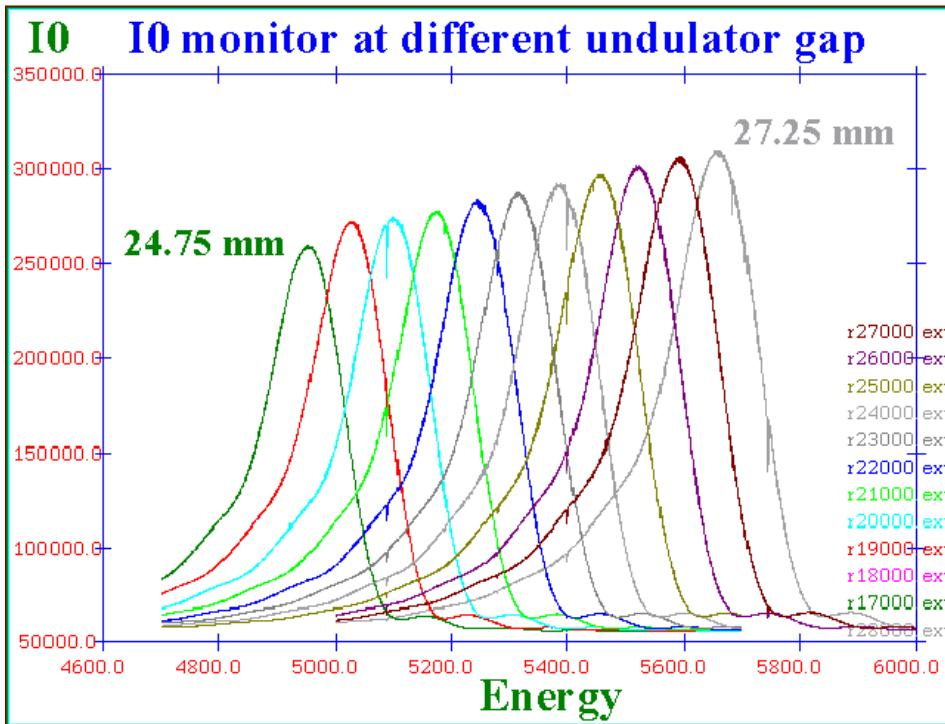
If the flux is to be maximized all while scanning the energy, the undulator gap must change as the energy is scanned.
