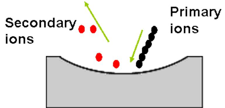
**Dynamic SIMS** : Top few monolayers are removed because of sputtering caused by the high dose of primary ions
