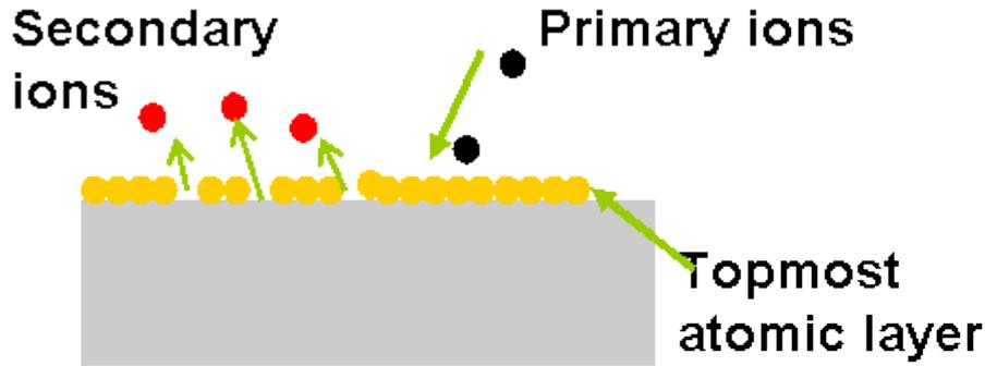
**Static SIMS** : Secondary ions are ejected only from the topmost atomic layer
