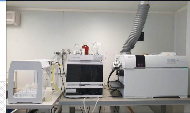
ICP-MS For Rare Earth Elements' analysis
